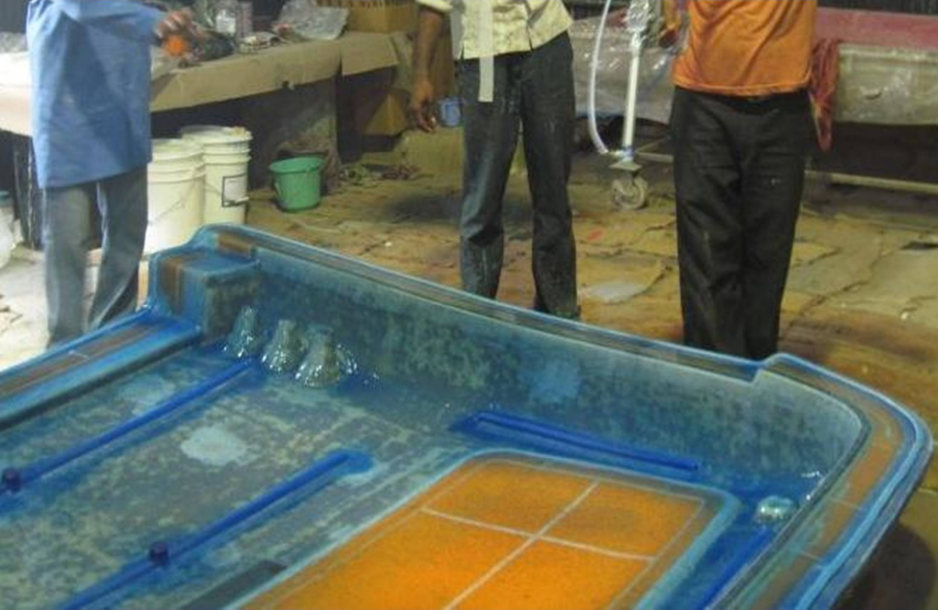
SILICON SPRAYING STAGE ON THE CALIBRATED FACE TOOL
